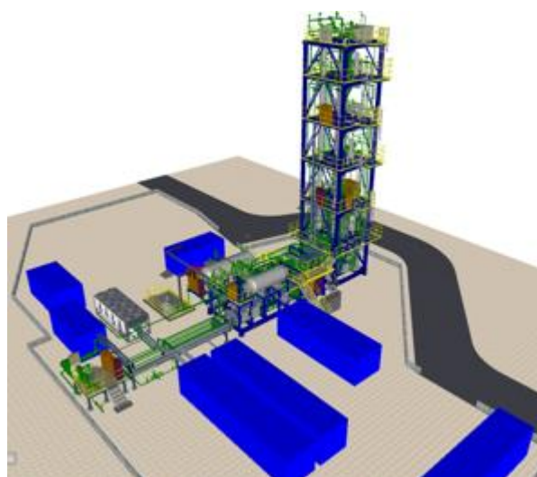
Figure 32: 3D Model of the Pilot Plant (Credits Axens&Artelia Group companies (France)) (Hamidian et al., 2021)
